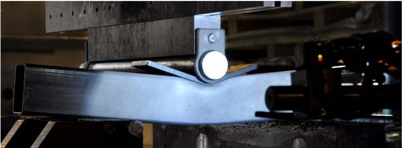
Figure 8. Optical strain analysis in bending of a beam
