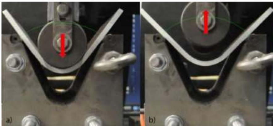
Figure 4. Bending of a steel plate in a V-die: a) punch in lower position; b) punch released
