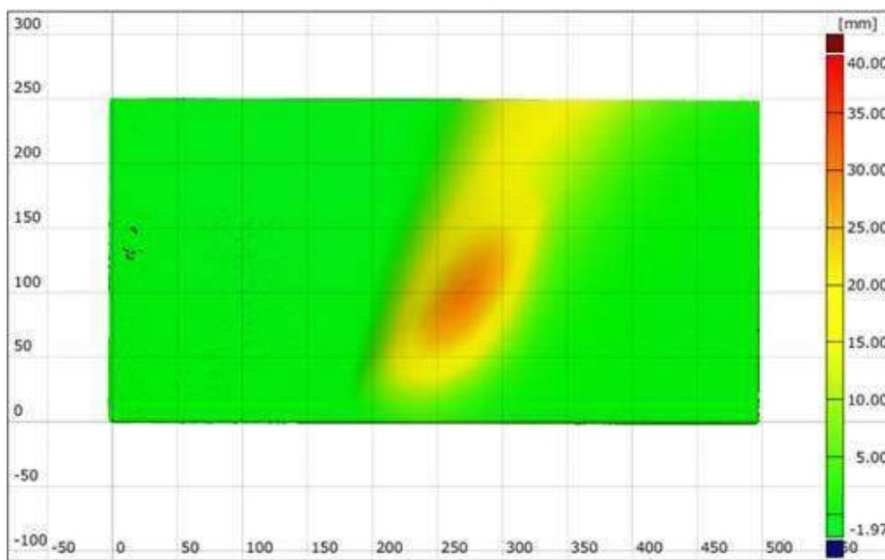
Figure 12. Wearing of side plate
