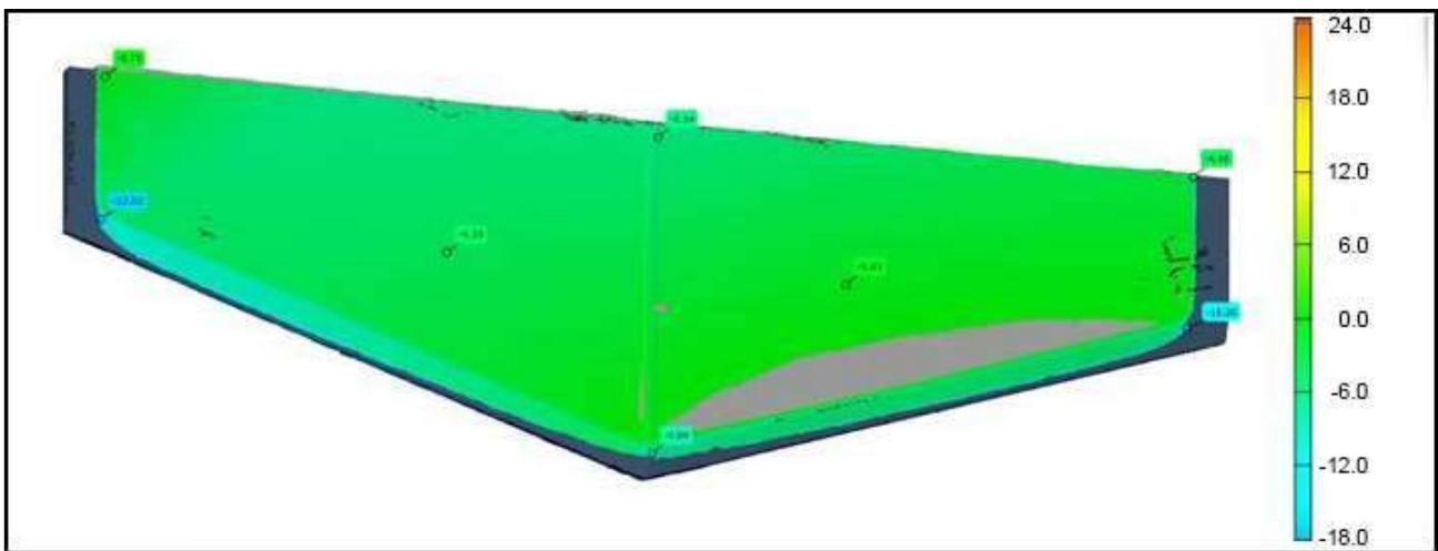
Figure 11. Wearing of cutting edge
