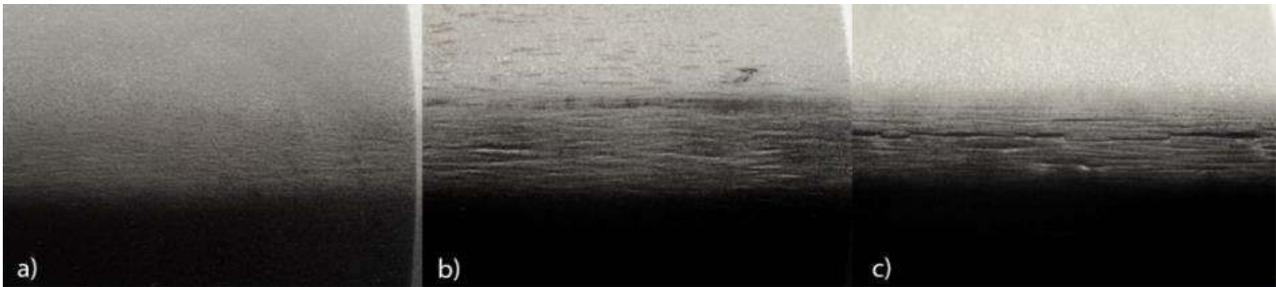
Figure 5. a) No failures; b) and c) failures appeared in the steel as a result of too small a bending radius
