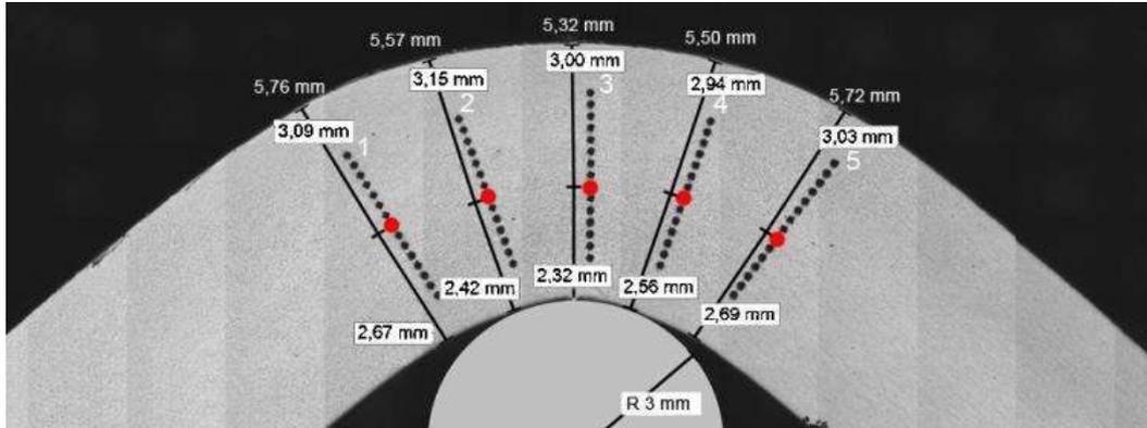
Figure 7. Microscopic image of the cross-section of the bend. The neutral axis is marked by red points based on the hardness measurements
