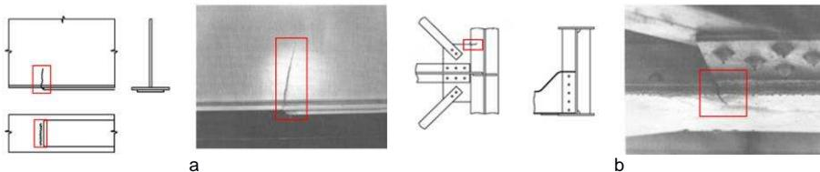
Figure 3: a) Fatigue crack at the end of a welded steel plate; b) crack in a difficult-to-reach area of a gusset
