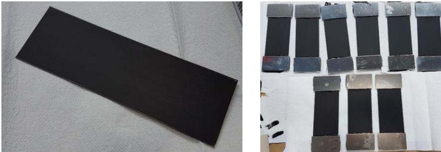
Figure 8: Specimen (left) and prepared specimens (right)
