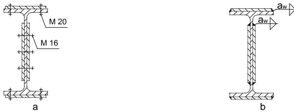
Figure 1: Example for conventionally reinforcements of steel girders with a) screwed and b) welded steel plates
