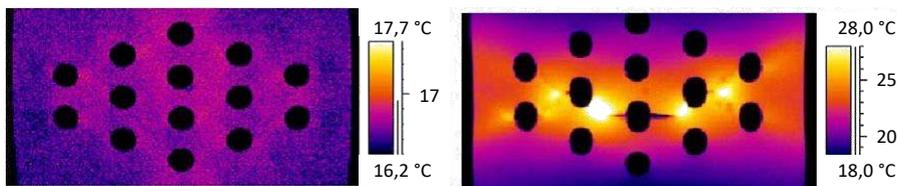
Figure 6: Temperature development of a tensile loaded specimen with holes at test beginning (left) and ending (right) (Müller 2005)
