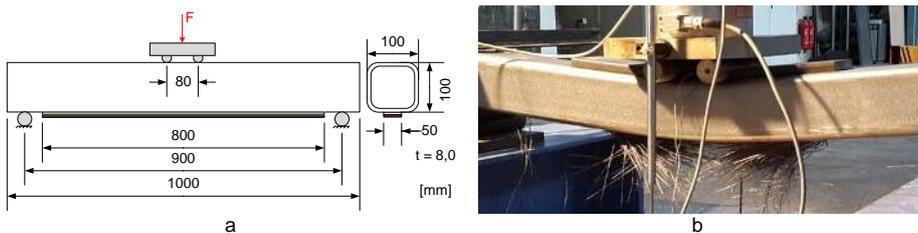
Figure 2: a) Test setup: hybrid reinforcement made of CFRP laminate; b) failure of CFRP laminate during testing
