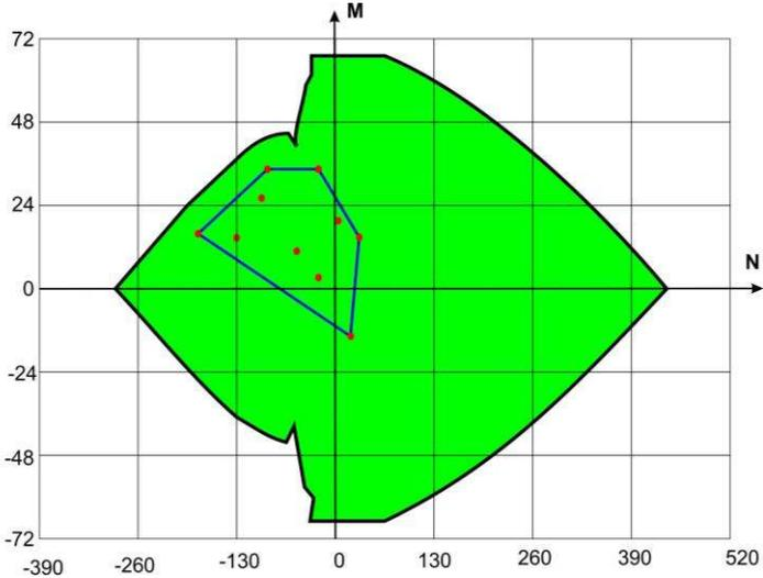
**Figure 9** Given (basic) loadings and their convex hull, combined with the load-bearing capacity area of the section
