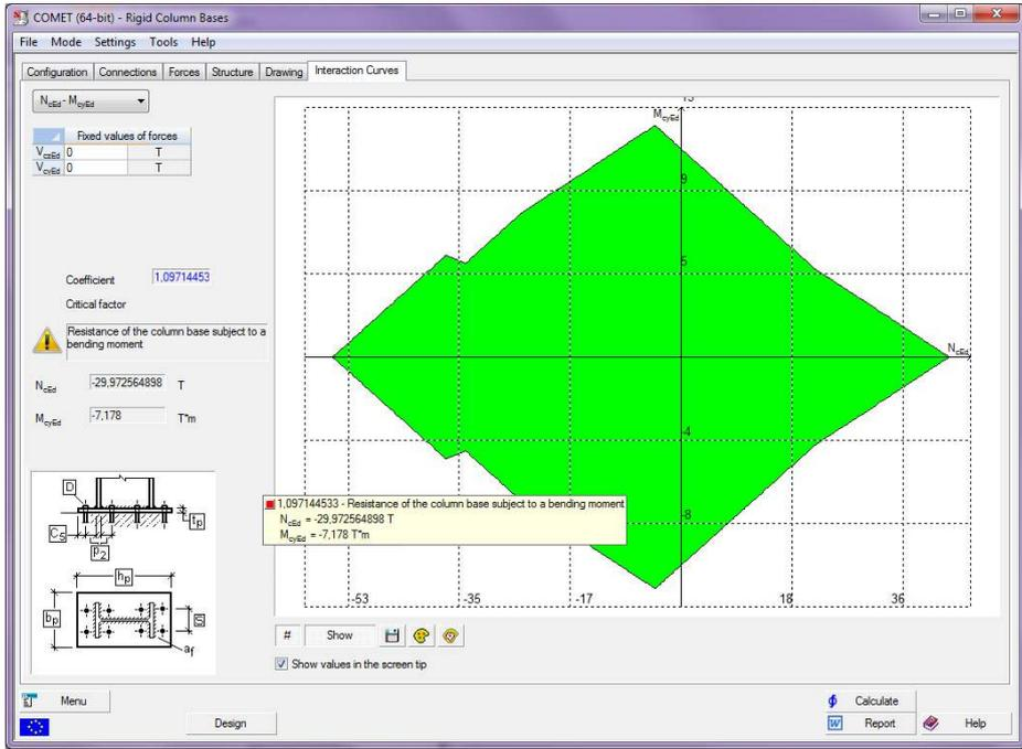
**Figure 8.** The load-bearing capacity area of the rigid column base using an equivalent reinforced concrete section when calculating the stress distribution in the foundation concrete and the forces in the anchor bolts
