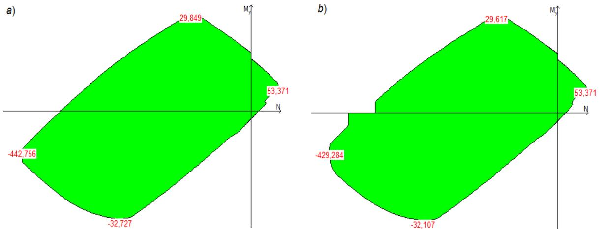
**Figure 7.** Effect of random eccentricity on the shape of the projection of the load-bearing capacity area of a reinforced concrete section
