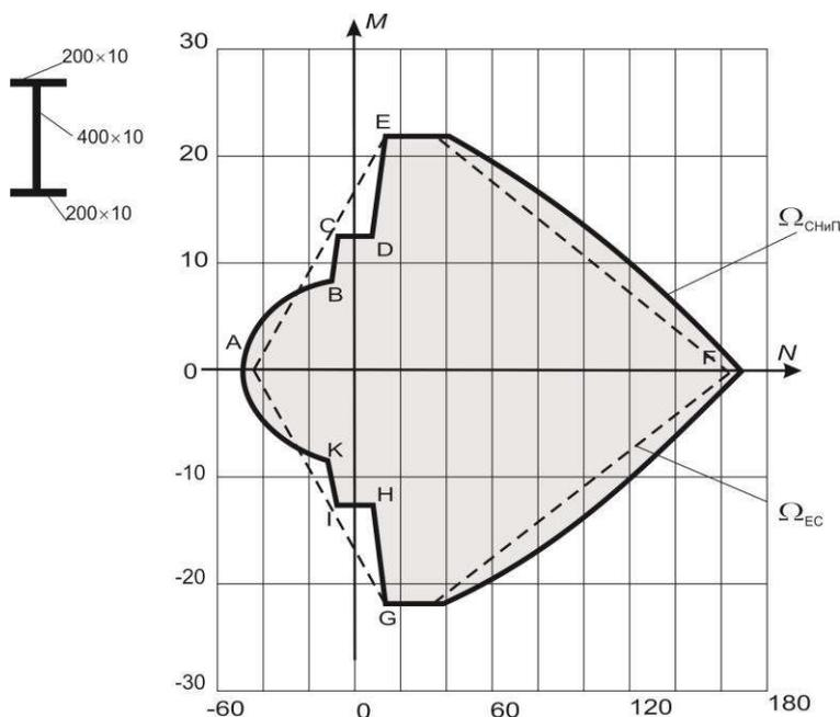
**Figure 5.** Load-bearing capacity area of a steel section:  $\Omega_{\text{SNiP}}$  – according to SP 16.13330.2011 (SP 16.13330.2011 2011);  $\Omega_{\text{EC}}$  – according to EN 1993-1-1:2005 (EN 1993-1-1:2005 2006)
