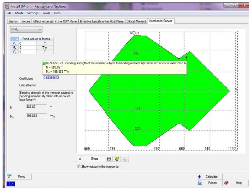
**Figure 4.** Interactive mode of exploring the load-bearing capacity area of the section
