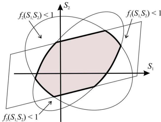
**Figure 1.** Formation of the load-bearing capacity area of a section in the two-dimensional space of internal forces (example)
