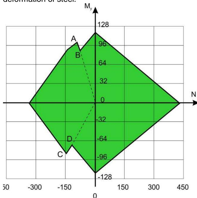
**Figure 6.** Load-bearing capacity area of a steel section according to EN 1993-1-1
