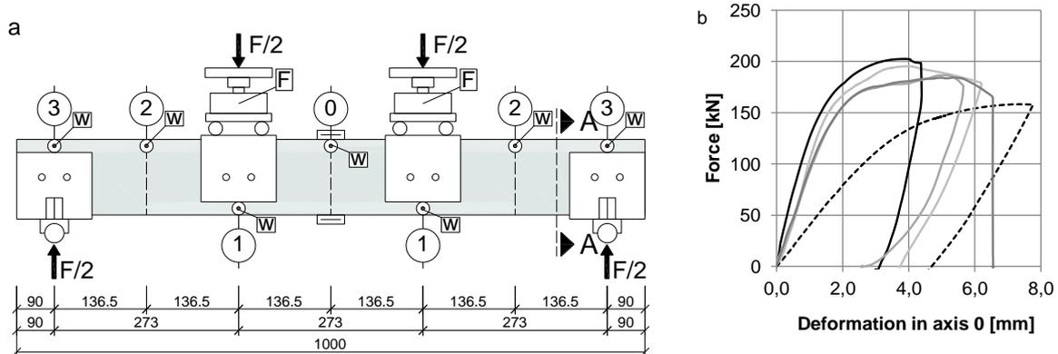
Figure 4: (a) Four point bending test; (b) Test results.
