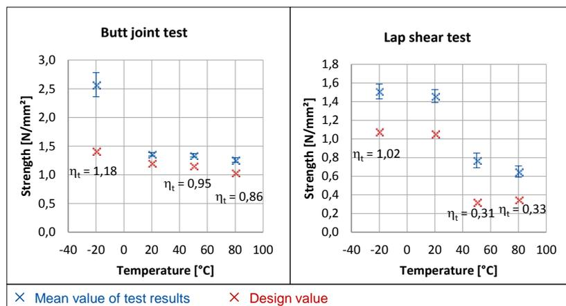
Figure 5: Conversion factors for a MS polymer adhesive
