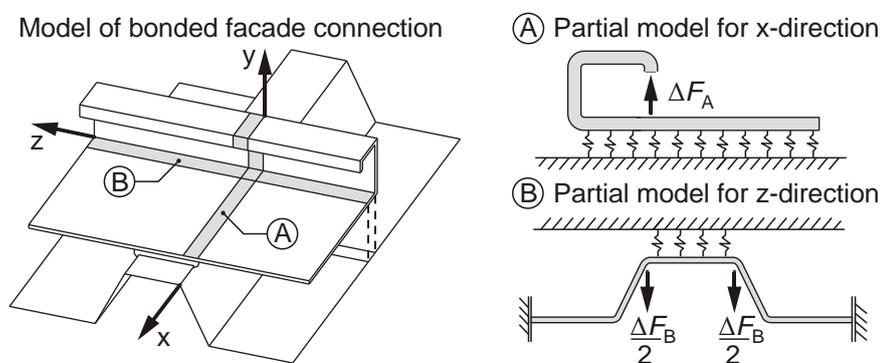
Figure 2: Model for the bonded façade connection
