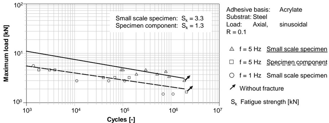
Figure 6: Comparison of test results of cyclic tests
