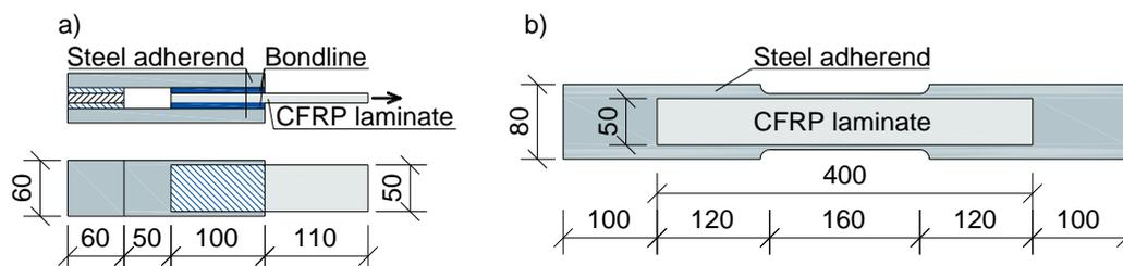
Figure 7: (a) Double steel-CFRP laminate-assemblies; (b) dumbbell specimen
