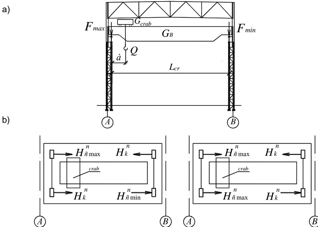
**Figure 1 – Schemes of crane loads:**
