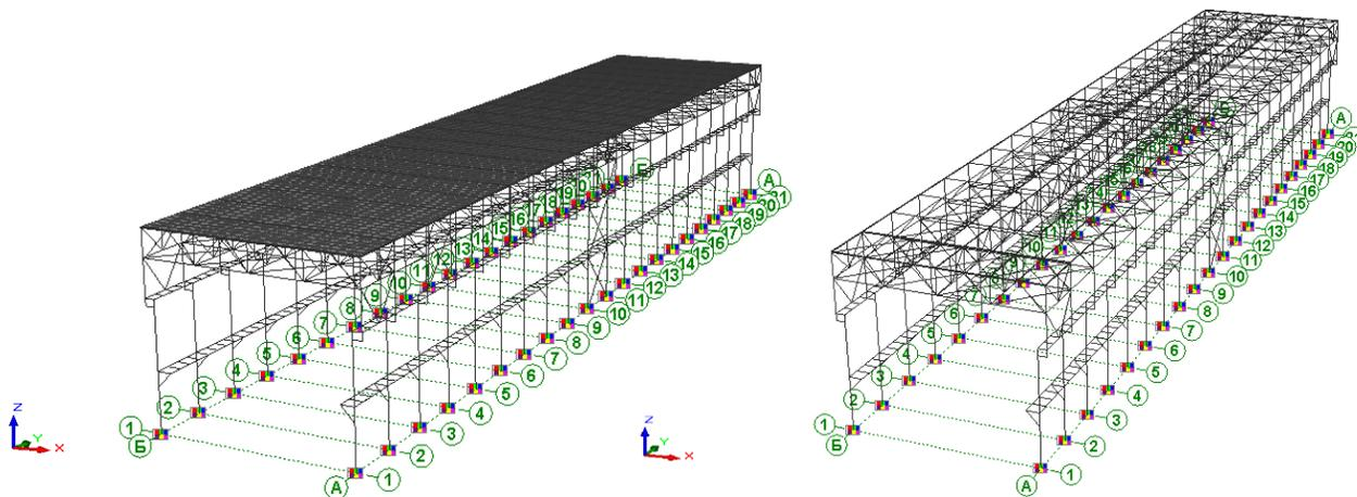
Fig. 2. Spatial design models of industrial building: a) with a «heavy» coverage (prefabricated concrete panels); b) «light» coverage (profiled steel on purlins)
