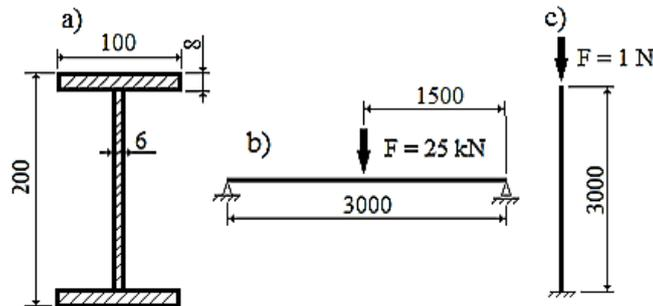
Figure 2. Objects of research: cross-section of investigated models (a); setting boundary conditions (b, c).
