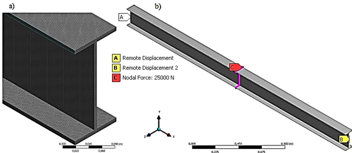
Figure 3. To the calculation of the rod for bending: the fragment of the partitioning of the I-beam into finite elements (a); boundary conditions (b).
