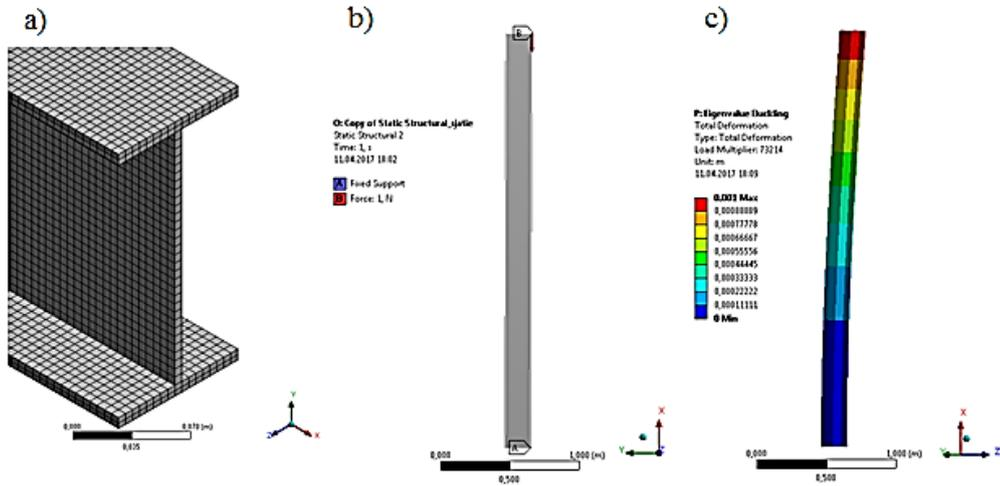
Figure 5. The results of the calculation of the rod for longitudinal bending, (type of SOLID): a) fragment of the partitioning of the I-beam into finite elements (a); boundary conditions (b); form of loss of stability (c).
