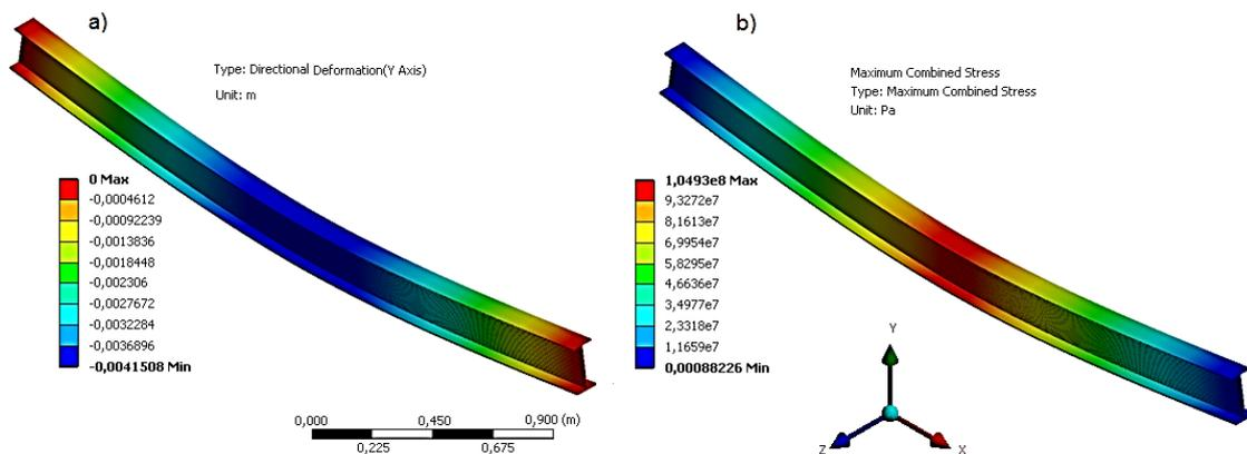
Figure 4. Results of the calculation of the rod for bending (FE of the BEAM type): deflection a); normal stresses b).
