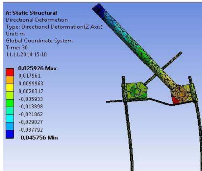
Figure 3 - The deform shape of the solid model
