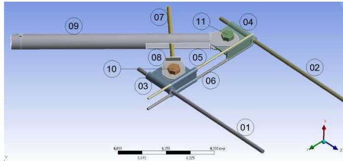
Figure 7 - The solid model, 01-Left Threaded Bar, 02-Right Threaded Bar, 03-Slider, 04-Span Bar (base), 05-Span Bar (Upper rod), 06-Span Bar (Bottom rod), 07-Support Rod, 08-Support Rod (base), 09-Lever Arm, 10-Left Bolt, 11-Right Bolt
