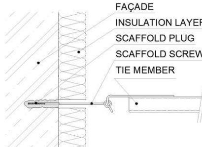
Figure 1 - Vertical section of the plugged anchor – because of an insulation layer a long screw is used
