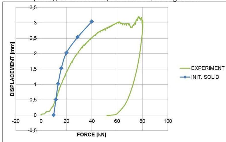
Figure 8 - Force – Displacement curve of the initial solid model
