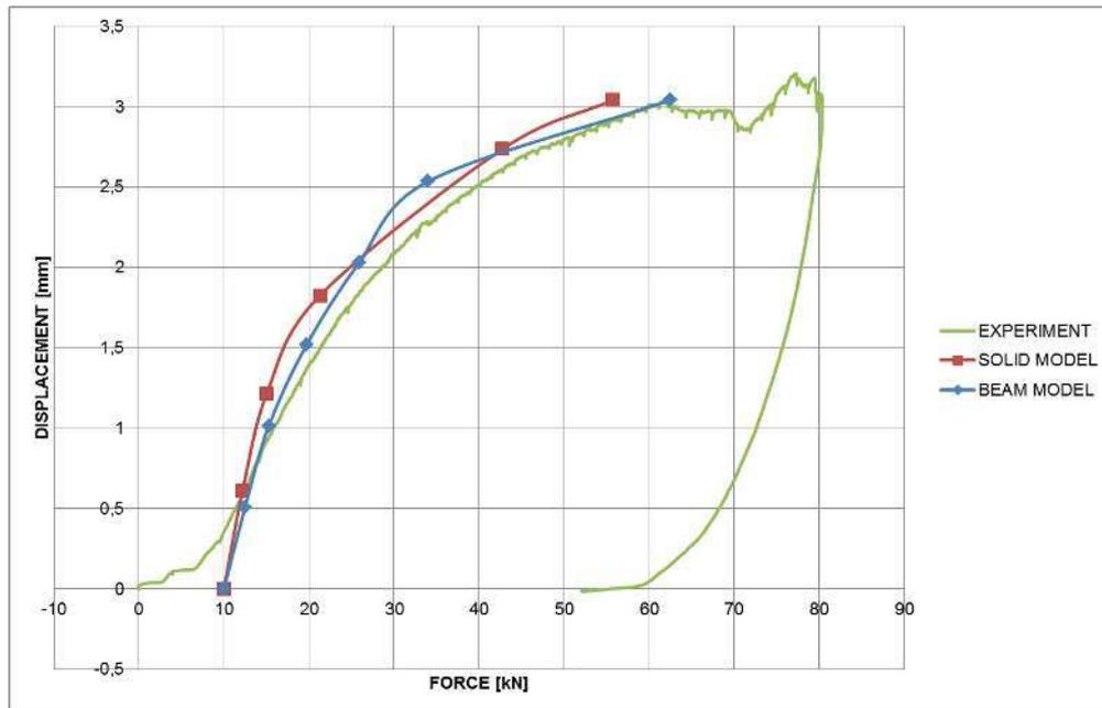
Figure 9 Force – Displacement curve and the deform shape of optimized models
