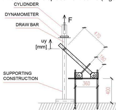
Figure 3 - The vertical section of the laboratory experiment
