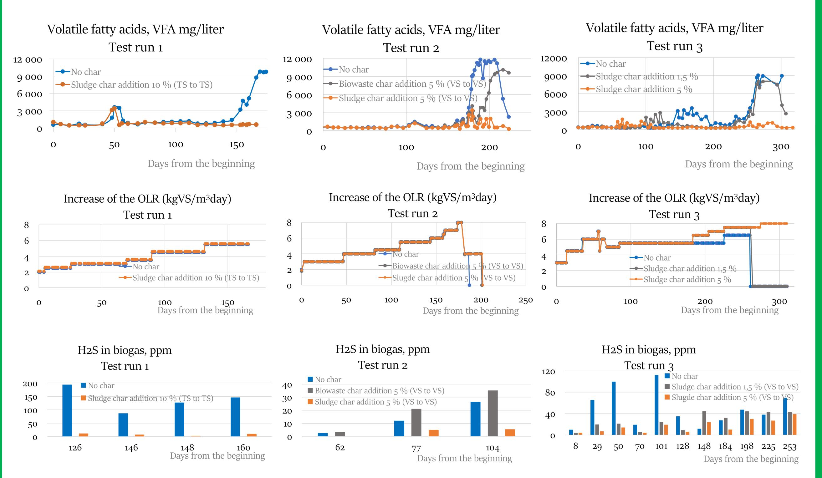
Based on VFA results, sludge biochar addition clearly increased the stability of the AD process of municipal biowaste. An addition of 5 % of sludge char to AD process was efficient enough while 1,5 % was not. No effect on methane content of biogas was observed while H<sub>2</sub>S concentrations were lower following sludge biochar addition. A high Fe content in sludge char probably limited H<sub>2</sub>S concentrations in biogas.
